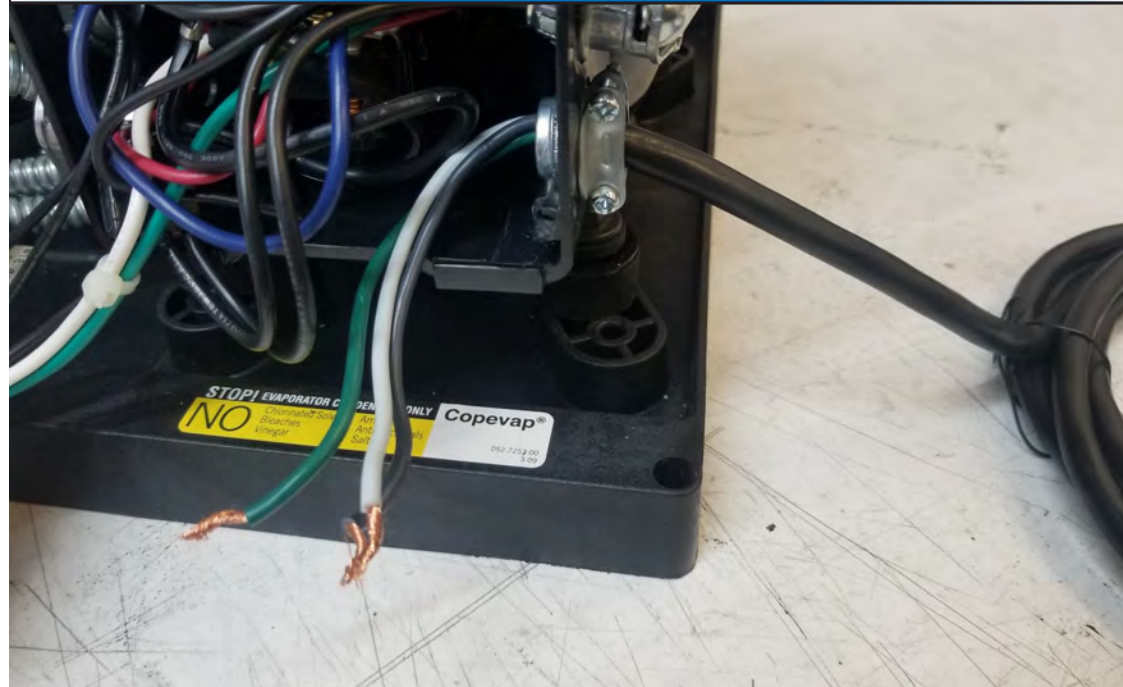
Route the required 115V power wires into the open clamp on the enclosure.
